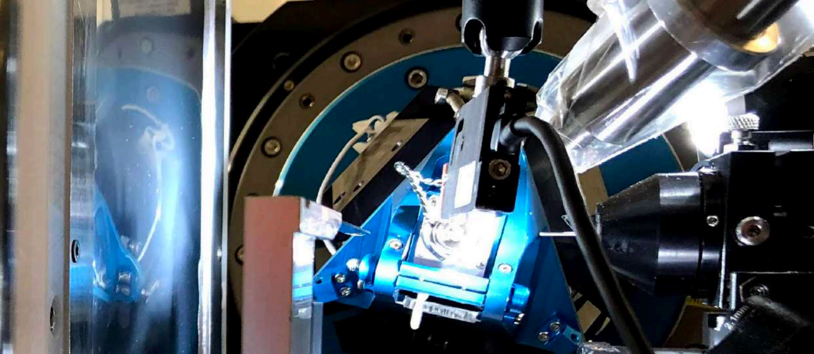
Set-up of the novel Jungfrau detector during tests at the beamline | ©PSI/Vincent Olieric
